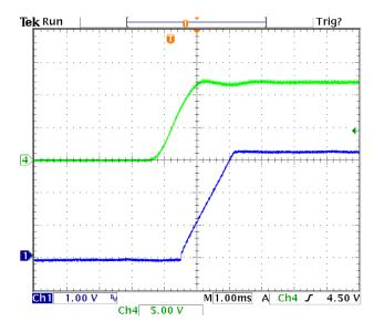
Figure 8. Typical Start-Up with application of Vin (Vo = 3.3Vdc, Io = 50A). Ch1 – Vout, Ch2 – Vin
