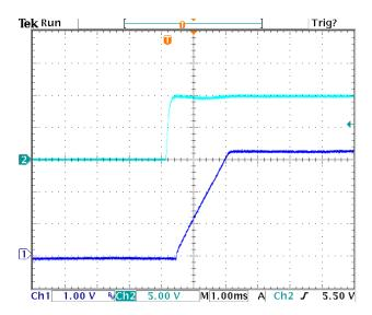
Figure 6. Typical Start-Up Using Remote On/Off (Vo = 3.3 Vdc, Io=50A). Ch1 – Vout, Ch2 – ON/OFF
