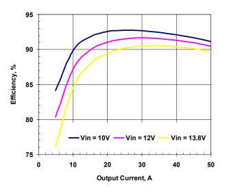
Figure 3. Efficiency vs. Load. Vout=2.5
