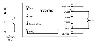
Figure 17. Circuit Configuration For ON/OFF Function
