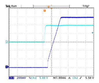
Figure 5. Typical Start-Up Using Remote On/Off (Vo = 1.2 Vdc, Io=50A). Ch1 – Vout, Ch2 – ON/OFF
