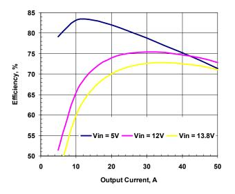
Figure 1. Efficiency vs. Load. Vout=0.6V
