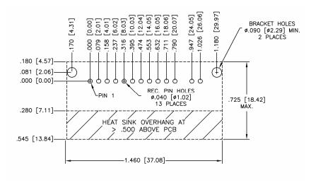
Figure 21. Recommended Footprint - Top View
