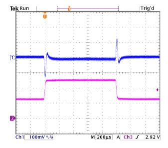
Figure 10. Transient Response to Dynamic Load Change from 50% to 100% of full load (Vin=12V, Vo=3.3Vdc). Ch3 – lout
