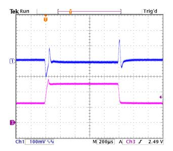
Figure 9. Transient Response to Dynamic Load Change from 50% to 100% of full load (Vin=12V, Vo=0.6Vdc). Ch3 – lout
