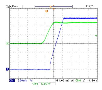
Figure 7. Typical Start-Up with application of Vin (Vo = 1.2Vdc, Io = 50A). Ch1 – Vout, Ch2 – Vin
