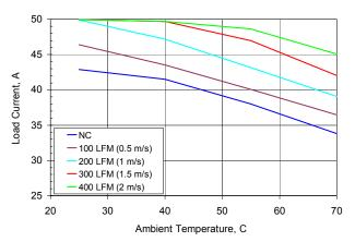
Figure 11 Output Current versus Local Ambient Temperature and Airflow (Vin = 12.0 Vdc, Vo=0.6Vdc)
