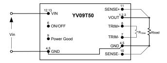
Figure 16. Programming Output Voltage With A Resistor
