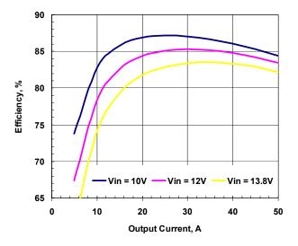
Figure 2. Efficiency vs. Load. Vout=1.2V
