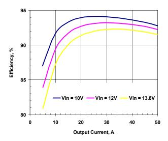
Figure 4. Efficiency vs. Load. Vout=3.3V
