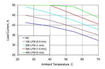
Figure 12. Output Current versus Local Ambient Temperature and Airflow (Vin = 12.0 Vdc, Vo=1.2Vdc).
